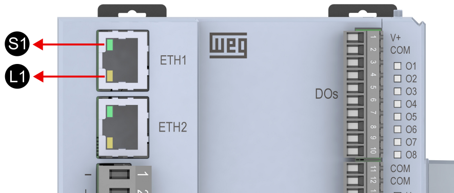
Figure 2.2: Speed (S1) and link/activity (L1) LEDs of the Ethernet interface of PLC500.
