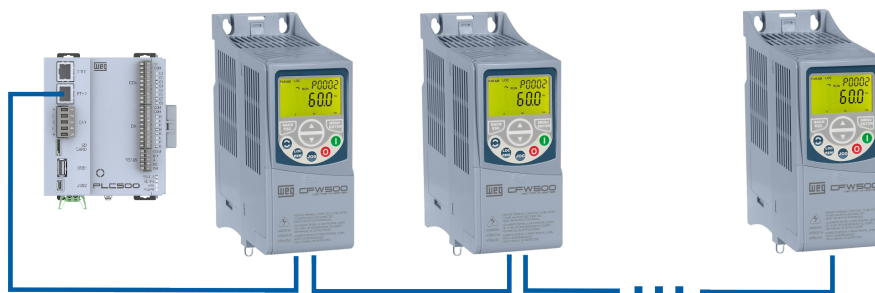
Figure 2.4: EtherNet/IP Daisy-Chain Topology.
