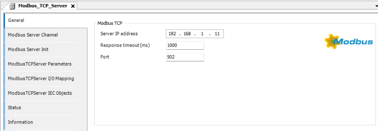
Figure 4.4: Network configuration for the server device.
