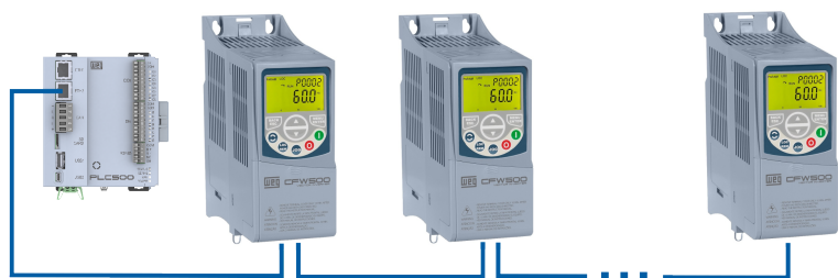
Figure 2.4: EtherNet/IP Daisy-Chain Topology.
