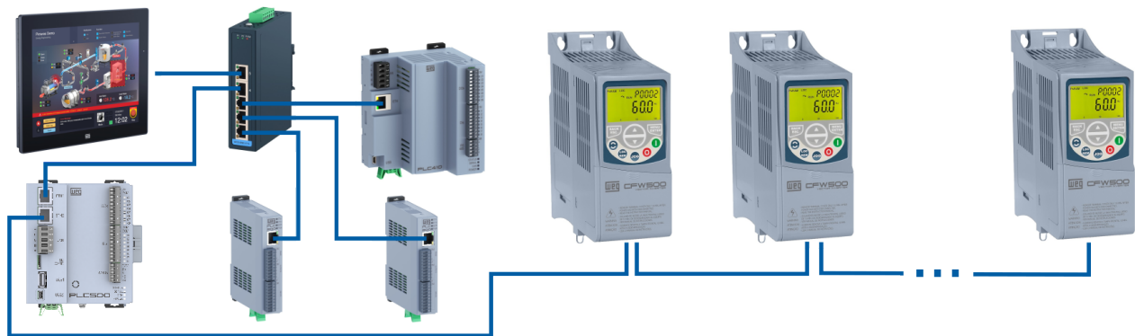
Figure 2.5: EtherNet/IP Star and Daisy-Chain Topology.
