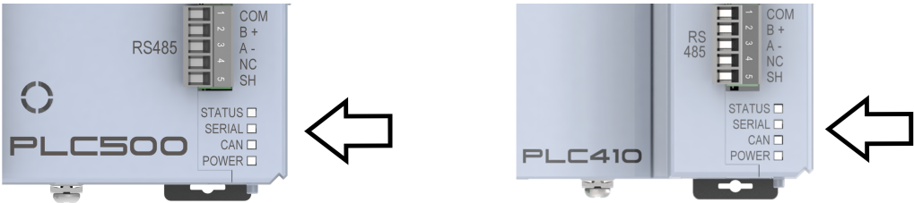
Figure 2.2: Indicator LEDs of the PLC500 and PLC410.
